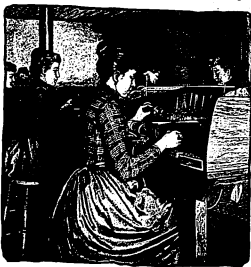
Fig. 20.—Sealing the Glass Socket and Carbon Filament into the Neck of an Incandescent Lamp.
